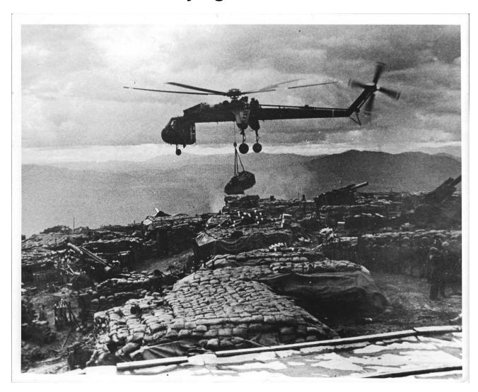
Other missions for the 355<sup>th</sup> Workhorses included recovery of downed aircraft (e.g. A1-E Skyraider, CH-47 Chinook, CH-34 Choctaw, OV-1 Mohawk), delivery of single point loads of 4 each 500 gallon fuel blivets (about 7 ½ tons), 175" gun replacement tubes (one of the heaviest and trickiest loads at 9+ tons), and numerous one-off unique requirements. In 1969, Workhorse Operation totals included 5,496 flight hours moving 34,620 tons of cargo.
