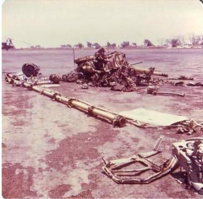
Wreckage of CH-47B 66-19106. Shown is the reassembled main drive shaft.
