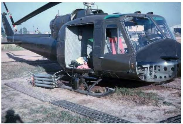
HU-1A with rockets and M-38, .30 cal. MG all installed by the UTT
