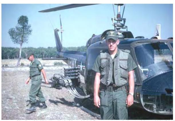
Charlie with HU-1B tail #21876 (which I flew on many missions) with quad M-60 MG's and UTT installed rockets
