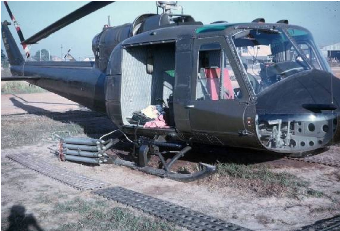
HU-1A (Huey) with UTT installed M-38, 30 cal. MG, and 2.75 inch rockets.
