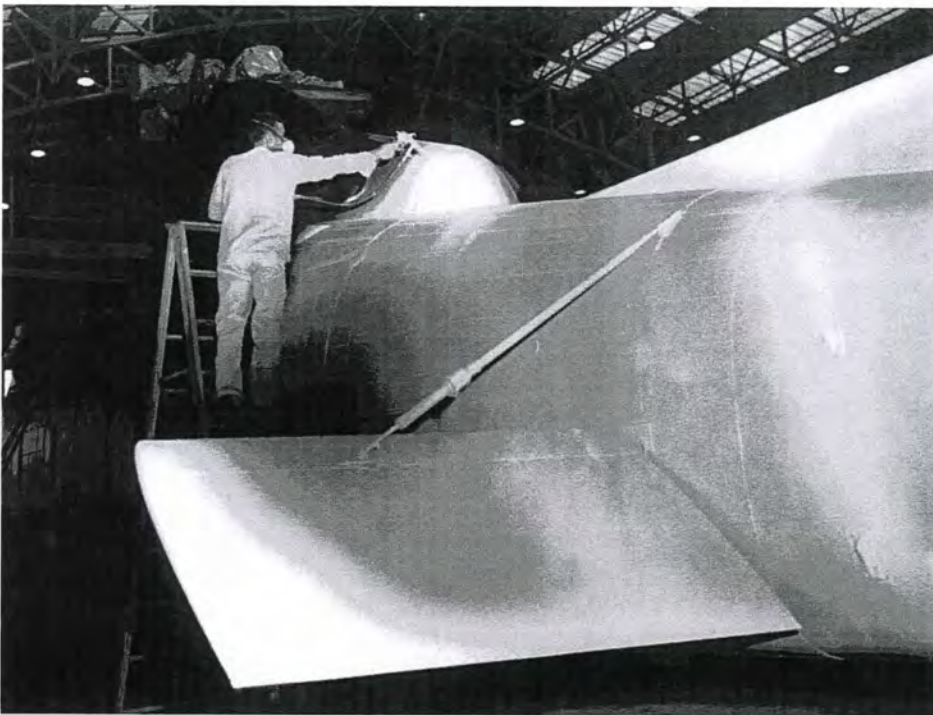
"CH37's receiving weather proof protection, before sea bound transportation, to overseas assignments".
